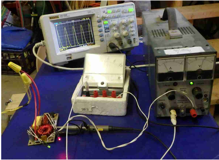
The test setup used for tuning. The oscilloscope shows the Class-E drain waveform. The loop was hanging 5 ft off the floor.
